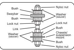
Fig.1. Whiteline double pin type link.
