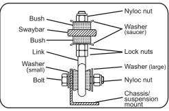
Fig.2. Whiteline pin/eye type link.
